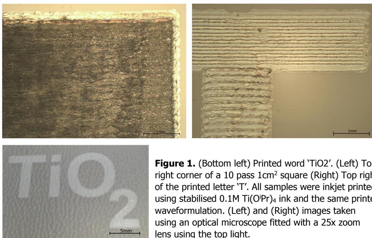
**Figure 1.** (Bottom left) Printed word ' $\text{TiO}_2$ '. (Left) Top right corner of a 10 pass  $1\text{cm}^2$  square (Right) Top right of the printed letter 'T'. All samples were inkjet printed using stabilised  $0.1\text{M Ti}(\text{O}^i\text{Pr})_4$  ink and the same printer waveformulation. (Left) and (Right) images taken using an optical microscope fitted with a 25x zoom lens using the top light.
